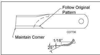
Figure 14. Blade Sharpening
